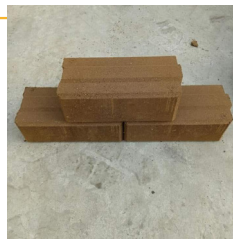
Hydraform Soil Interlocking Block (9by x 8by 115mm)
