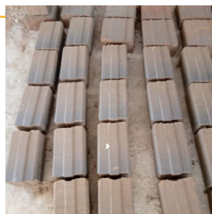
Standard Soil Interlocking Block (200mm x 115mmx100mm)
